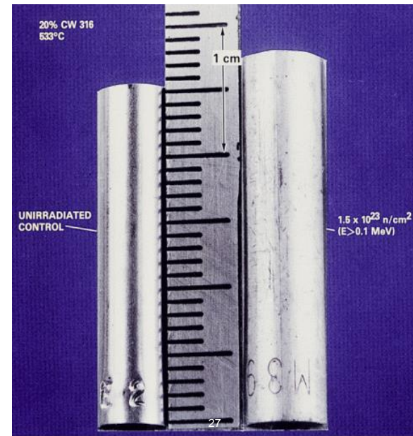
Radiation swelling of 316 stainless steel [4]
